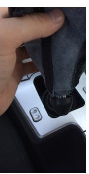
**3.** Line up 4 fins on shift knob with slots inside retainer nut. Press 2 parts together. Place shift knob/shift boot/retainer nut on shift lever. Push up and rotate retainer nut counter clockwise until snug.
