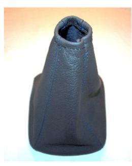
**9.** Slide new boot over shifter shaft. Position the top of shifter boot just above plastic ring. Do not pull boot over white plastic ring on shaft as in original installation.
