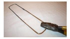
**16.** The new Redline e-brake boot has a channel sewn into the base to receive the wire retaining ring. Find an opening in this channel and carefully feed the ring all the way around the boot base until the ring is completely inside the channel. If needed, move the ring around inside the channel so the front and back stitched seams are located at the small ends of the rectangle. The boot is now ready for installation.
