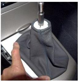
**12.** Pull the e-brake lever up to engage the emergency brakes. This will provide the clearance needed to remove the boot. The base of the stock boot is held in place by four plastic clips below the surface of the counsel opening, on the left and right side. With your fingers, pull right side of the base of the boot to the left, away from the right side of the counsel to unclip.
