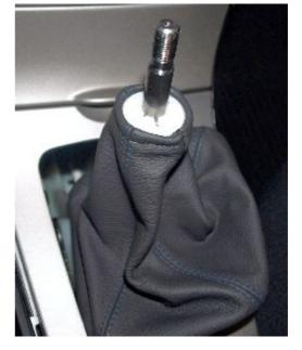
**10.** Snap retaining ring in place on base trim plate. Wider end goes toward the front of the car.
