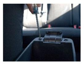
**20.** Remove the two screws holding the armrest to the hinge and remove the armrest
