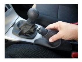
**18.** Slide it down inside the counsel opening by turning the base slightly and while holding at an angle, lower into the counsel. Then work the base up and into the two clips on the left side of the counsel. Pull the right side of the base up and into the two clips on the right side of the console.
