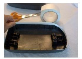
**27.** Remove the non-stick paper from the tape and fold the tape over the edge and down the inside of the cover. Place the armrest top centered over the new cover. Push down on the back end of the armrest to compress the padding enough to allow approximately 1/4" (6mm) of the leather to overlap the edge of the armrest. Fold over the carpet tape to attach.
