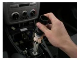
**9.** 9. Notice the staples on the base of the old shift boot that secure it to the plastic boot bracket. Remove the staples by prying them out with a flathead screwdriver.
