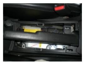
**3.** Once the bezel is loose, you must disconnect the electrical connectors to the accessory input by the e-brake and the cigarette lighter by pushing down on the clips and pulling out at the same time.
