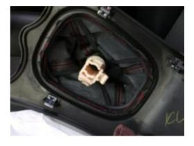
**13.** Put the bezel back into place and reconnect the two electrical connectors and push the bezel in to secure it.
