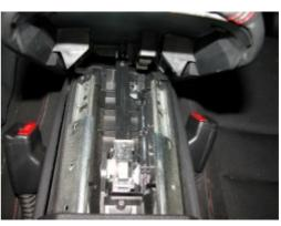
**10.** Unscrew the six screws on the underside of the armrest and pull of the plate holding the fabric in place.
