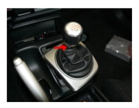
**2.** Push the boot down into the console and grab the inside rim of the silver trim piece and pull up evenly on both sides. It should pop right off.
