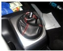
**3.** There are 4 torx head screws holding the boot to the silver trim piece. Remove the screws and pull the boot and ring out through the bottom.
