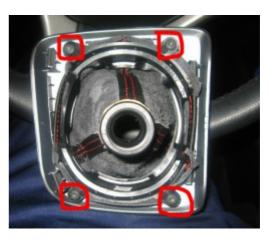
**4.** The boot is secured to the ring with 6 staples. Remove them with a pair of needle nose pliers or anything else that might work.
