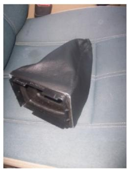
**6.** Invert the boot and with a straight razor or a sharp knife, carefully cut the first rung of the old accordian style boot completely around the inside.
