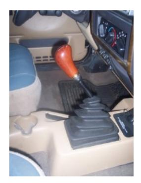
**2.** Once the shifter is removed, remove the old boot and bracket by simply pushing in the front end (the side nearest the emergency break) until you can remove the bracket.
