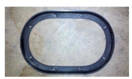
**9.** Place upper half of bezel over top of shift boot and line up bolts with holes in shift boot.
