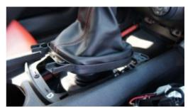
**8.** Under the retaining ring, you'll see holes where fabric from the boot is pushed through. There are small teeth in each of these holes keeping the material in place. A good tug will free the fabric from the teeth. You can also use a small flathead to carefully push the material through if desired.
