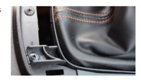
**7.** The boot now lifts easily off with the attached retainer ring.
