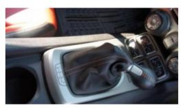
**3.** Remove the shift knob from the silver cap on top of the boot. As with step 2, it takes some force but will come off.
