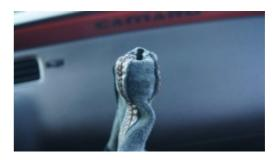
**12.** Insert the silver cap into the new boot. Make sure that you slide the silver cap into the new boot upside down! This will be much tighter in the
