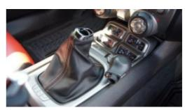
**4.** Lift the top of the center console. It's easy to separate and lift with bare fingers. A trim removal tool or a very small flathead screwdriver may also be used.
