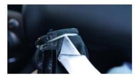
**10.** Turn the boot inside out. There is a zip-tie keeping the material tight around the sliver cap at the top. This will need to be cut.
