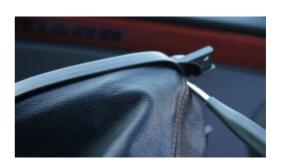
**15.** Use a small flathead screwdriver to push the leather into the teeth on the plastic ring.
