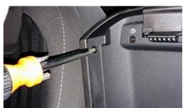
**3.** Remove the top section of the arm rest cover from the console. If all the screws have been removed, the piece should come right off without having to apply any force.
