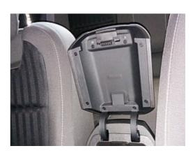
**2.** Remove the 8 retaining screws from the arm rest.
