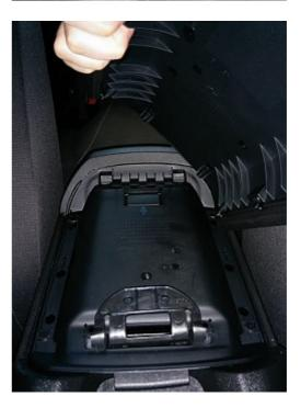
**4.** Thoroughly clean the surface of your arm rest before applying any adhesive. If your original cover already has a leather wrap, it will have to be removed before any other step is taken.
