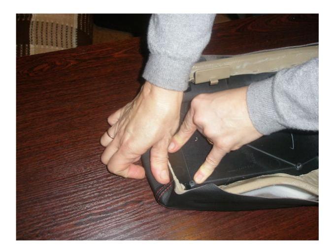
**8.** Make small cuts in the cover around the dip to allow leather to align around this concave curvature well. Stretch and glue around the edge of the dip.
