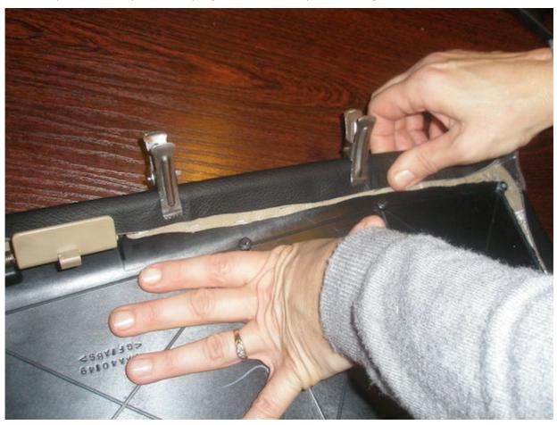
**11.** After the glue has settled (check glue container for directions and necessary setting time designation), reassemble the armrest.
