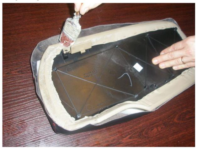
**7.** Pressing down on the armrest, to compress the foam, pull the leather and glue it around the edges. Start with the front, do the rear next, and the sides last.
