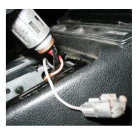
**6.** Pull the power feed straight off of the lighter. (On some cars, it may be necessary to unscrew the lighter assembly to remove the grounding ring).
