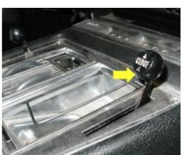
**3.** To remove the shift knob, simply unscrew counterclockwise.
