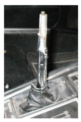
**4.** Pull the reverse actuator straight up, be careful not to lose the spring.
