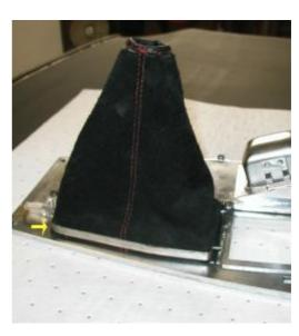
**9.** On some vehicles, it may be neccessary to remove the 4 screws holding the ashtray in place to get the shift boot over the shift plate. Replace the ashtray as soon as the boot is installed.
