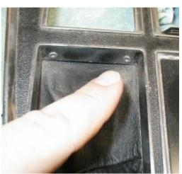
**8.** Turn the new boot inside out, pull it over the shift plate, and pull the collar over it.
