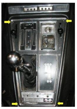
**2.** Use a 1/16" allen wrench to loosen the set screws holding the Astro Vent knobs in place. It is not neccesary to remove the said screws completely. Put the knobs and screws in a safe place.
