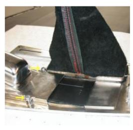
**10.** Reinstall the 4 screws hold ing the boot and collar on.
