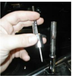
**5.** Remove the light from the ashtray lighter by squeezing the sides together gently.
