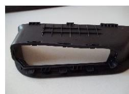
**16.** Carefully separate the two parts and at the same time, remove the boot (only clipped between black and grey parts) and keep parts apart.
