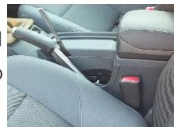
**12.** Carefully poke the knife between the center console and the cover around the boot and carefully pry it apart.
