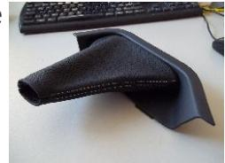
**19.** To refit into car, you'll have to try two different ways. As seen here, carefully pull it over the brake lever/handle. This can get a little tough, as the handle gets wider towards the bottom and can possibly tear seams on the boot. If you find it difficult, try the version below.
