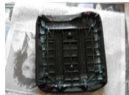
**10.** Now wait 30 seconds then put the cover on top of the leather. Now press down on the edges. To avoid wrinkles make sure you pull on the leather from opposite sides. Do it everywhere and check the back to make sure there are no wrinkles. Binder clips will be very helpful in making sure the fitment is tight. Once glue dries, reinstall it into the car.
