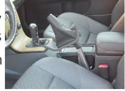
**20.** Put a thick (unprinted) plastic bag over the handbrake and thread the boot over the plastic bag. I found this easier because the bag cancels out the friction between the handle and the boot...
