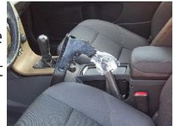
**21.** Clip the plastic trim into the center console and get the seam around the end of the brake lever straight.
