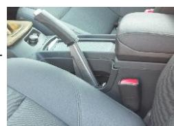
**13.** E-brake boot is only removable after removing the whole cover, pulled up and over the brake lever.
