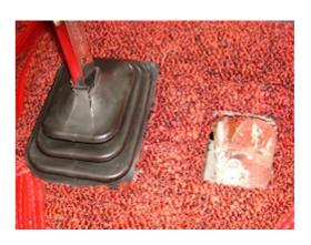
**10.** Replace cover plate, nut and shaft ball on shift console.
