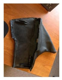
**10.** Inspect the boot to make sure all edges are properly secured. To reinstall into the car, reverse steps 1-3, slipping the new boot over the handle and pushing the clips down into place (this may require some added force with the leather option as it is now a bit thicker overall.)
