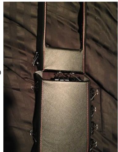
**13.** Begin gluing the fabric to the passenger side trim and hold in place with clips while it dries. Again, you may have to trim small pieces of fabric as you go to avoid folding and gathering. Remove your clips after the glue dries and clip back into place in the dash.
