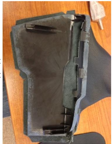
**6.** Apply contact cement or any industrial adhesive to the front and the edges of the plastic frame on the back side.
