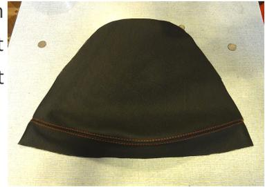
2. Test-align the cover on the gauge hood, make sure it fits perfectly before you even start glueing
