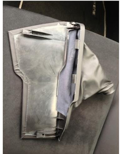
**5.** Carefully peel the stock vinyl from the plastic frame by lifting it up from the corners. The stock adhesive is not too strong and it should come off fairly easy without tearing.
