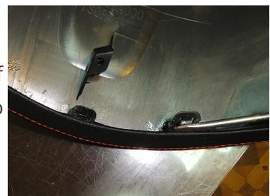
**13.** It might help to use a screwdriver, putty knife or even a ruler to make the glue hold the leather along the clips.
