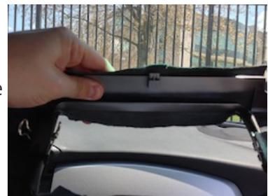
**8.** Cut a notch out of the fabric to allow for it to wrap around the clips in the middle of the trim piece.
