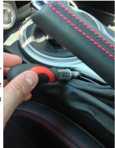
**2.** Lift up carefully to release all of the clips. Pull the bezel up.
