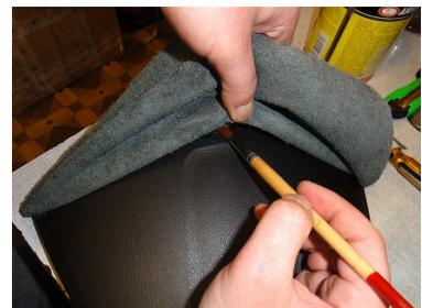
**10.** Then proceed with applying the glue to the upper surface of the hood making sure you apply the glue to the whole surface - lift the leather a bit and slide the brush under it to spread the glue in there. You can glue the whole surface at once making sure to spread the leather evenly. Do not stretch the leather too much.
