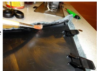
6. Then apply the glue to the bottom surface of the hood cover along the front edge, fold the leather and press it strong to make it stick to the glue. Make sure the leather holds tight especially at the clips areas
