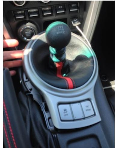
**3.** Using a flat head screwdriver, release the clip holding the traction control button harness into the bezel. Unscrew and remove the shift knob.
