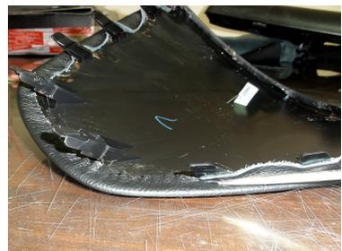
**16.** You will need to make small cuts in the leather on both sides of every clip to make it lay properly.
