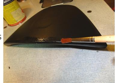
3. First glue the driver-facing edge of the hood - apply the glue along the edge with a brush - approx. 1-2cm to both sides of the edge.
