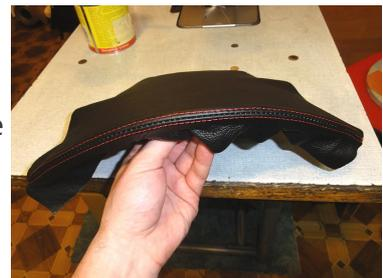
5. Make sure it's nice and tight, seam properly aligned to the edge and let the glue settle a bit.
