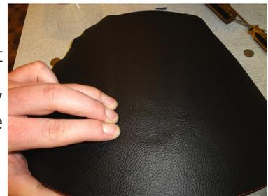
**12.** Let the glue settle and then apply the glue to the bottom of the hood along the edges, fold the leather and press firmly to make it stick.
