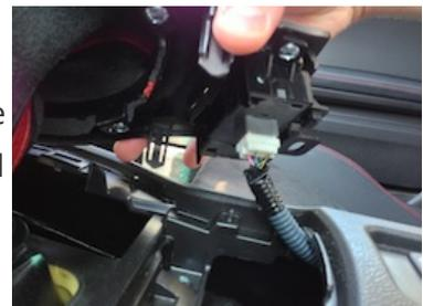
**4.** Unscrew and remove the shift knob. Carefully pull the stock shift boot up and over the reverse lockout to remove the assembly. Remove the 4 screws holding the boot frame to the bezel to and remove it
