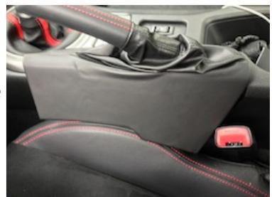
3. Lift the assembly up and slide the fabric up and over the brake handle. It will slip over it and the boot assembly will now be free.
