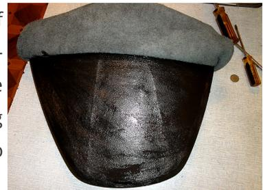
**11.** Instead, before you lay it on the whole surface, press it strongly into the hollow to make the leather stick there, (otherwise it may lift there after some time) and then press the leather firmly all over the surface till the edges.
