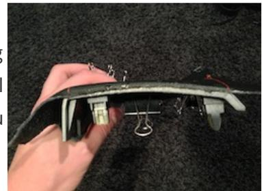
**12.** Clip the fabric to the passenger side dash piece and line it up with the stereo trim to be sure the stitching lines up.
