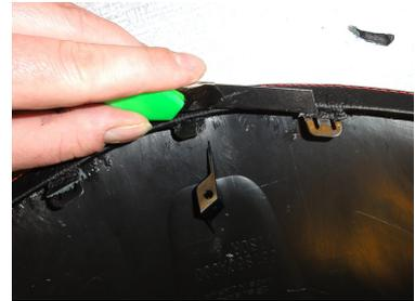
**9.** ... including trimming the leather just a bit to make it sit flush.
