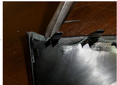
**17.** After the glue settles firmly cut the excess of the leather that lies on the clips in order to make the clips snap back into the dashboard.
