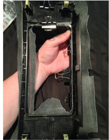
**11.** Begin gluing the edges of the fabric to the trim piece using industrial adhesive or contact cement. You may need to cut small pieces of fabric off to allow for it to wrap around curves as you go. replace the clips as you glue to create a good bond.
