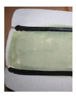
**2.** Carefully remove the cover, but be careful not to damage the underlying foam. In the ends, it gets very thin and will likely stick to the cover.
