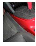
**6.** Remove the cover by peeling it starting from underneath. Be careful not to tear the foam under that cover, since it may adhere to the cover. Align the material to the pad, paying special attention to the circular cut at the front end. Mark it in pencil if necessary.
