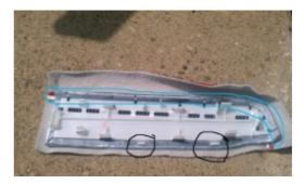
Glue the armrest on. You can use contact cement, a spray-on glue that will give you a while to do the final adjustments before it settles fully is recommended.
