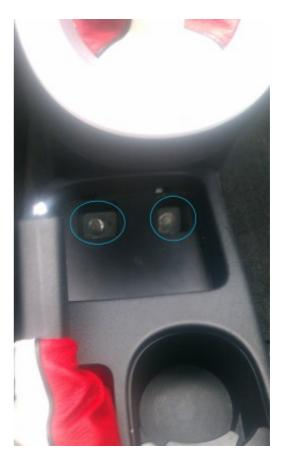
open the arm rest and use your flathead to remove the bottem of the compartment as you did the fron and remove these bolts.
