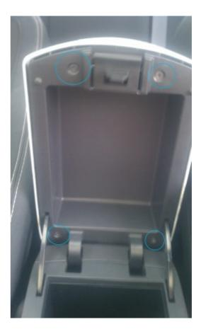
**6.** With this off you can slip the leather cover over it and glue it down to the rubber cover already on yours. There was no modification required here. Just make sure everything stays tucked and glued. With the console closed put the newly covered lid over it and press down to make sure it all goes on properly. Mine was a nice tight fit. Then open it up and hold pressure on the back to put the screws back on the inside of the lid.
