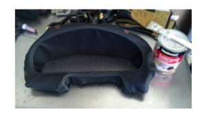
**4.** Take some time to get a plan of attack and an idea of where the leather will want to bunch or pull away. Then get started with the cement. I chose to do the flat upper panel first and clamp it in place until everything was dry. That allowed me to get the seam lined up and know that it wouldn't move later on.
