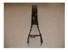
because the boot won't reach reach the final 2 at the front. Turn the new boot inside out. Using the rubber as a guide, make slits about 8mm or so long corresponding to each button, about 5 mm from the edge of the boot. Use the slits to mount the boot with the buttons between the rubber gasket and the console.
