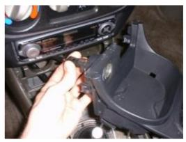
**3.** To remove the stock shift boot, pop it out from the clips that hold it into place.
