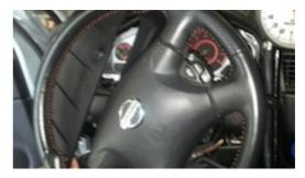
**3.** The wrap will come out of the box and lay over the factory plastic panel. You will need some clamps and contact cement:
