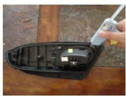
**13.** As you can see, there is some melted plastic on the top end of the cup (where the arrow is pointing). This initially keeps the cup from being pried away from the rest of the armrest. This plastic "weld" can be snapped, if it wasn't done so from your initial removal. This will allow the leather to be pulled through.
