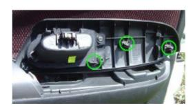
**12.** Glue will be necessary to temporarily hold the cover in place until it is fully installed. Hot glue allows for a good temporary bond to secure the cover to the arm rest.
