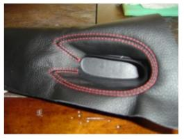
**16.** Flip the arm rest over and begin gluing the cover to the edges of the arm rest. Be sure to pull tight as you glue them.
