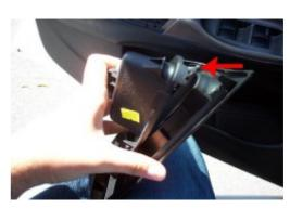
**14.** The cup cutout of the cover was pulled through and folded in between the cup and the rest of the arm rest. As you can see, hot glue allowed it to be held in place. Continue this process all the way around the cup.
