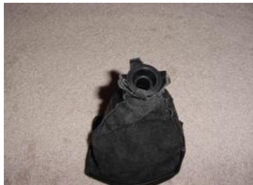
**5.** Turn the boot right side out, and insert the metal band into the boot. Try to line the band up with the folded over part on the boot.
