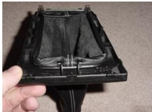
**9.** Remove the center console to fully expose the e-brake handle. To do that you need to remove 5 screws from console: 2 front, one under a small cover at the brake lever, 2 beneath the plastic cover at the rear by the cup holders. Then you need to pull off 2 plastic covers on each side underneath the dashboard, and the one around the cupholders, before taking the console up.
