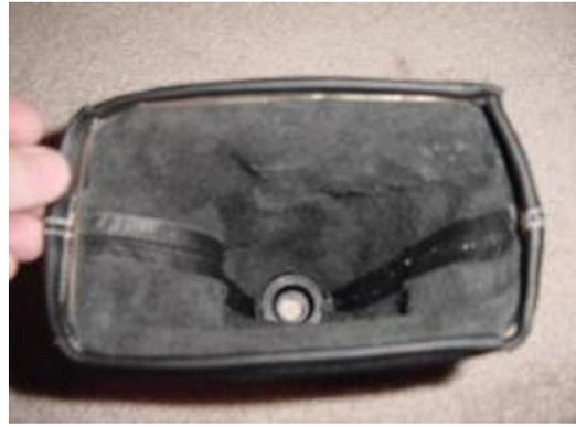
**6.** Look at the plastic trim. Notice the opening matches the metal band. Make sure to line the small end of the band up with the small end of the plastic trim.
