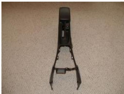
**10.** Pop out the rubber gasket surrounding the ebrake. Little buttons hold it on. We used only the 5 buttons from the rear down to hold it, because the boot won't reach reach the final 2 at the front. Turn the new boot inside out. Using the rubber as a guide, make slits about 8mm or so long corresponding to each button, about 5 mm from the edge of the boot. Use the slits to mount the boot with the buttons between the rubber gasket and the console.
