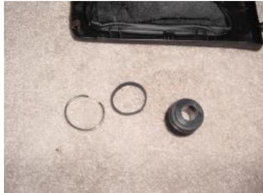
**3.** Next you need to remove the metal band from the old boot. Use a razor knife to cut the material. Here is the metal band removed. Notice the band is not a perfect rectangle. The smaller end faces the rear of the car.
