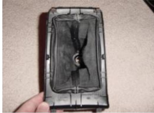
**2.** Turn the boot inside out, and remove the plastic cap, metal collar, and rubber band.
