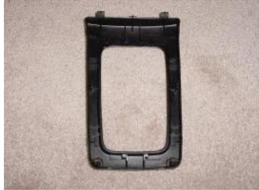
**7.** Now insert the boot into the plastic trim. Because the leather boot is thicker than the old one, it will be a tight fit. The boot will slip under the side clips, but not the front and back ones.
