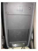
**8.** Then there are 3 more screws to actually separate the cover from the armest. Glue the new cover over the armrest, wait for glue to settle and reinstall.
