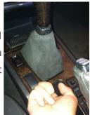
**3.** Now that the shift boot is un-clipped and free, it is time to remove the shift knob. Make sure the shifter is in neutral and pull straight up hard on the knob. You can also twist and wiggle the knob to help get it loose.
