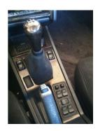
**2.** Get your finger below the wood console surface through that hole and undo the shift boot clips. They go all the way around the boot. Once you pop the back to clips you can pull the boot loose and off the shift boot retainer.
