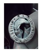
**8.** Align the new REDLINEGOODS shift boot on the black base ring. Clip the chrome trim ring onto the black base ring, sandwiching the boot between the two rings.
