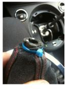
**10.** Clip the tail of the zip tie and wrap the zip tie with electrical tape to prevent tears in the leather.
