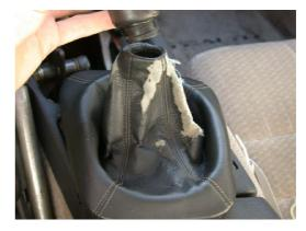
**2.** Remove the plastic zip-tie to separate the boot from the knob. We recommend a razor blade for this.
