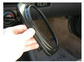
**4.** Here's were you need to be careful: Before making any slots in your new genuine leather shift boot for the shift plate hooks, place the shift plate within the boot and experiment with where you want to make the incisions. Note that the boot is customized for the 3000GT/Stealth, and as such, make sure the running edge is longer on the left than on the right. Depending on what look you
