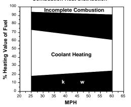
ly reduces the power output of the engine. Figure 1 shows a typical heat balance diagram for an internal combustion engine. This diagram demonstrates that the coolant in an internal combustion engine must absorb and reject through the radiator 2 to 3 times the amount of energy which is converted to brake power.
