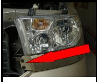
1.) Remove both black plastic rivets by prying up center portion with a flat head screwdriver.
