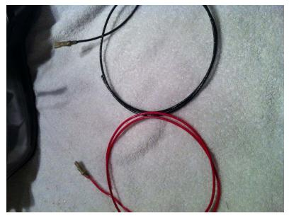
• STEP 4: USE 12" OF RED AND BLACK WIRE AND CONNECT FEMALE CONNECTOR TO ONE SIDE OF EACH WIRE
