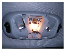
2) With the lens removed, unscrew the 3 Philips head screws completely to remove the housing from the ceiling. Once the housing is free from the ceiling, unclip the electrical power line and remove the center primary dome light bulb.
