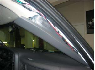
Route the harness down the PS pillar and thru the opening at the corner of the pillar. Some find it's easiest to route mechanic's wire first then use the wire to pull the wire harness down underneath the glove box right behind the connector panel.
