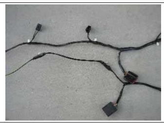
Here's a good comparison of the wiring harnesses. You see the additional nodes on the right picture. Those are for the clearance lights. You will have to remove the passenger kick panel and really fight the plastic rivets behind the glove compartment. They will finally give up the fight. You do not have to re-rivet the portion of the wiring harness that runs down the kick panel. It can be very difficult to get your hands in there.
