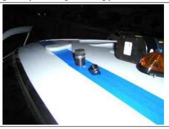
Then use a Knock Out (7/8") tool to make the center holes for the lights. The outer holes for the studs are drilled to 1/4" to provide some fudge room. Keep the shop vac hose handy to vacuum the shavings as you go along.
