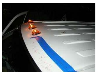
The last thing to do is pop the harness rivets back in place, put the headliner back up, visors, pillars and final clean up. And getting all the grease pencil markings off the roof!
