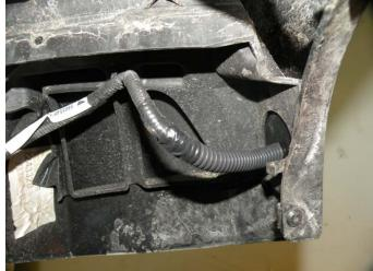
Re Install The Fender lining & The Plastic Buttons.
