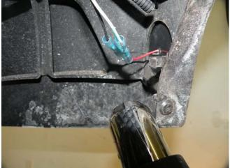
Using The Wire Loom Cover The Wires & Connectors.
