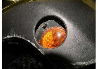
Push The Tab Down And Pull The Top Of The Lens
