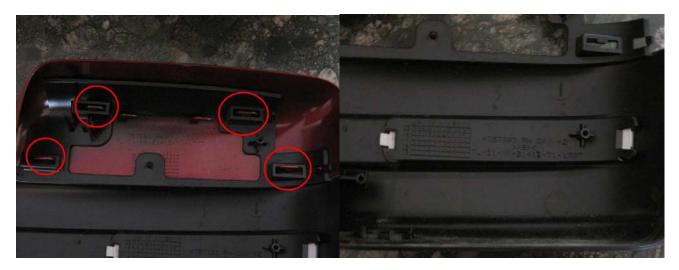
6. Now you can remove the reflector from the housing. Using a flat head screwdriver, gently pry the tab on the outside curved part of the reflector. NOTE: The driver mirror reflector tab on the door side is a fork shape instead of one solid tab.
