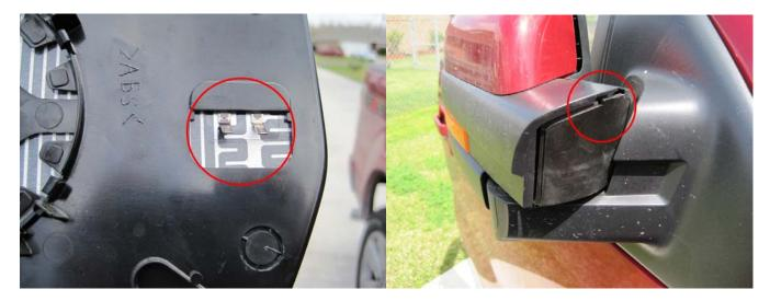
4. Now fold the mirror in towards the door of the truck so you can remove the front half of the housing. Start at the door side of the mirror and pry up as shown. Once you have this part up the housing should pop right off.
