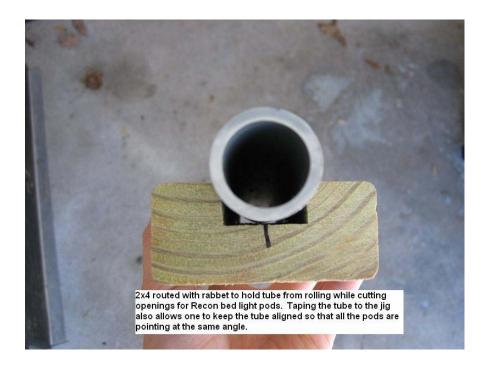
I then placed the tube, taped to the jig, on my radial arm saw equipped with a dado blade to make the holes for the light pods to stick through. You can cut these holes with a box knife or coping saw but a dado makes a much cleaner level cut.
