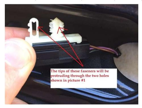
As shown in the picture, the two white clips hold the factory connector in place.
