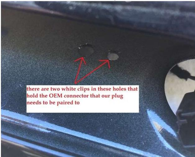
As shown in the picture, the two white clips hold the factory connector in place.
