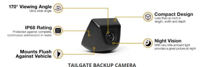
The Tailgate Backup Camera is built with an MT9V139 sensor and a lens with an ultra wide viewing angle of 170°. Its tiny size (less than an inch long, wide and deep) makes it ideal for smaller vehicles and allows its installation to be virtually invisible. It mounts flush against the vehicle and with an IP68 weatherproof rating is fit to operate in almost all weather conditions.
