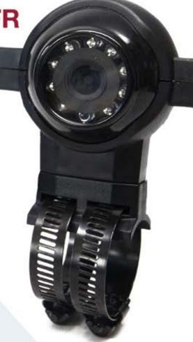
Keep it simple with the Freightliner Arm Camera. The RVS-ARM-FR is designed to fit this onto the arm bracket of your Freightliner truck, no drilling necessary! This mirror image camera is equipped with a wide 120° viewing angle, a 2.8mm lens and 10 infra-red lights for excellent night vision. Completely waterproof with a IP68 rating, this camera also has a 10G vibration rating.
