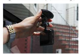
STEP 1: Mount Dash Camera on windshield behind rear view mirror.
