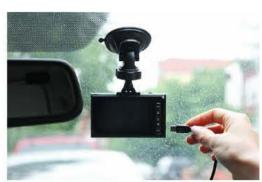
STEP 3: Attach power cable to the dash camera.
