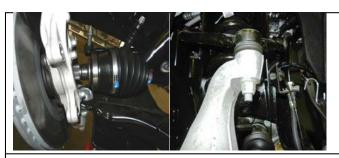
Reinstall the axle into the steering knuckle. Reinstall the upper control arm to the steering knuckle. Torque down using a 18mm socket. Install the factory hardware to the axle and tighten down with a 36mm socket. 17.
