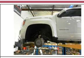
Lift the vehicle by the frame. Then remove the wheels using a 22mm socket.
