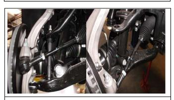
Remove the sway bar end links from the vehicle. Using a 15mm socket on top and a 13 mm socket on bottom.
