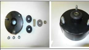
Install the rubber bushings to each side of the spacer. Lube the metal sleeve and press into the bushings. 14.
