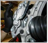
Unbolt the axle nut using a 36mm socket. Use a soft mallet or press tool to knock the axle from the knuckle. Remove the brake calipers from the 7. knuckle using a 18mm socket. Hang out of the way.
