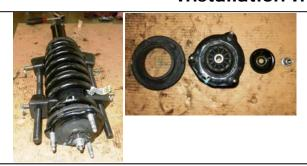
Once spring tension is off of the nut, remove the spring hat with a 15mm (nut) and 6mm wrench (shaft end). Remove the top hat and rubber isolator.
