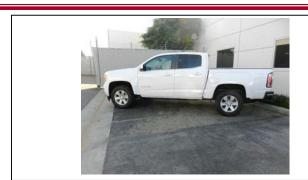
Put the vehicle onto level ground. Measure from the ground to the center of the fender well at all four wheels. Record the data in 1. the space provided on page 2.
