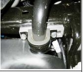
Install the sway bar offset spacers to the frame using the factory 10mm bolts. Install the sway bar to the offset spacer using the provided 10mm x 1.5 x 20mm bolts and a 14mm socket. 19.
