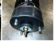
Install the rubber isolator and ReadyLIFT top hat spacer onto the strut using a supplied washer and gold 10mm x 1.5 flange nut. Use a 15mm and 6mm wrench. Make sure to line up the markings from top to bottom on the strut. Do not use an impact gun, tighten down by hand.
