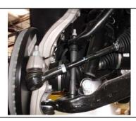
Reinstall the tie-rod using a 21mm socket. Reinstall the sway bar end links using a 13mm socket for the bottom and a 15mm socket for the top. 20.
