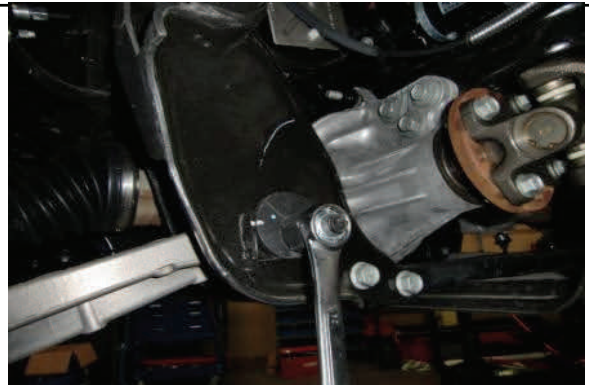
Mark and loosen front/rear lower control arm alignment cams
