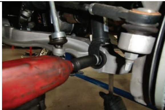
Remove lower strut mounting nut.
