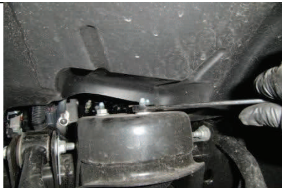
Now remove upper strut mounting nuts.
