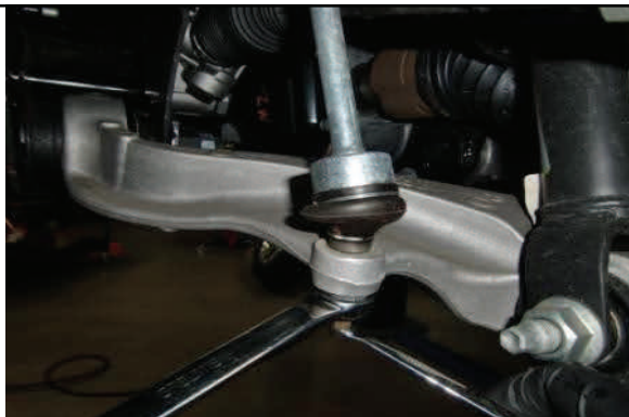
Loosen and remove lower sway bar nut.
