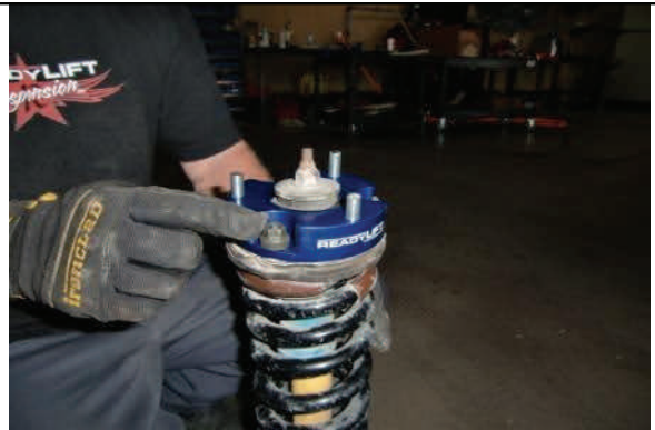
Attach assembled spacer to top of strut w/ OE hardware
