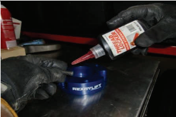
T6 Only Assemble billet spacer with thread locker
