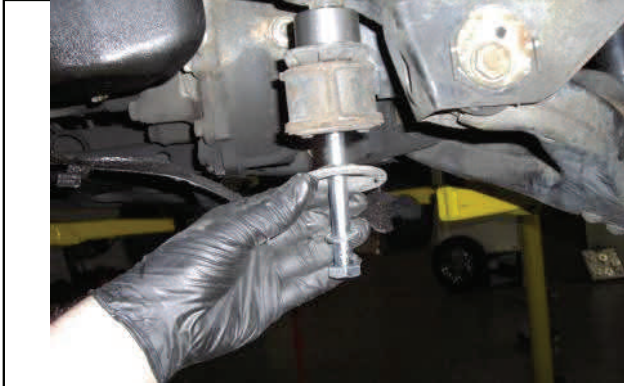
4WD Install longer bolts and reattach differential to frame
