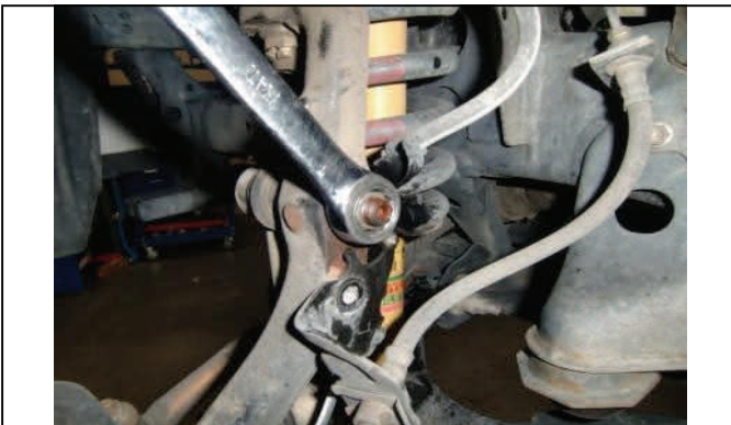
Disconnect sway bar end link at spindle
