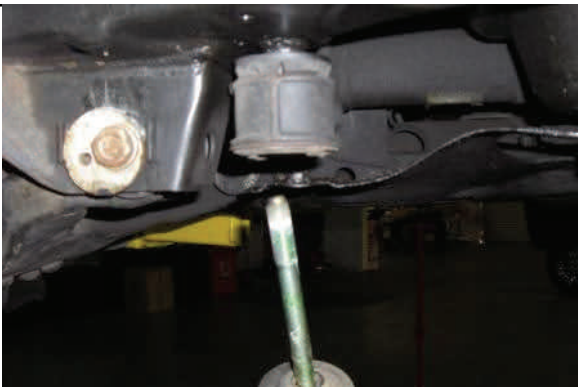
4WD Support differential & remove front mounting hardware
