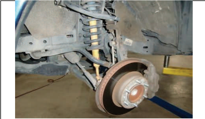
Raise and support vehicle on frame
