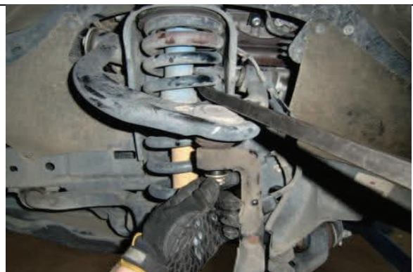
Support suspension and remove upper ball joint nut
