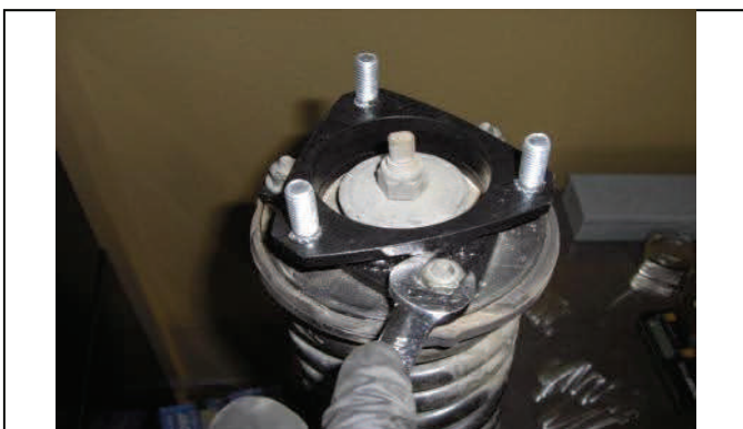
Attach new strut extension with OE hardware
