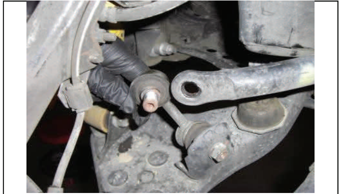
Disconnect both sides sway bar end links
