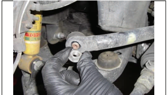
Reconnect sway bar end links. Move to the rear installation
