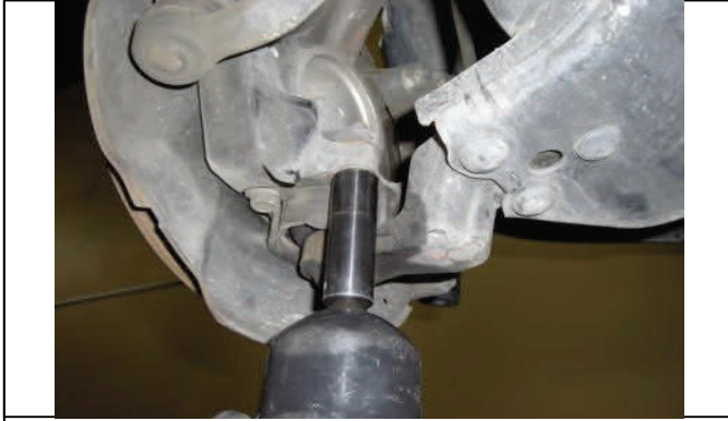
Reattach lower ball joint bolts and tighten
