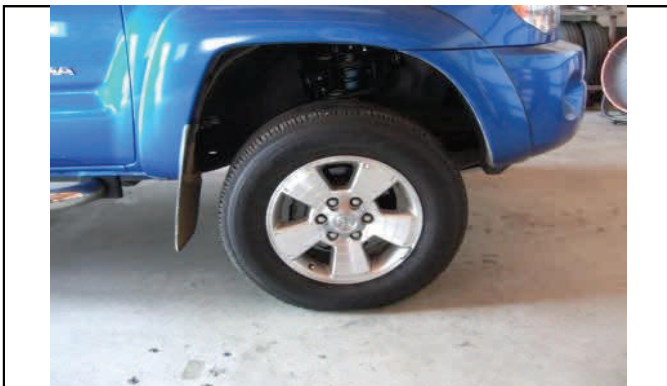
Reconnect sway bar links, install wheels/tires torque to spec.
