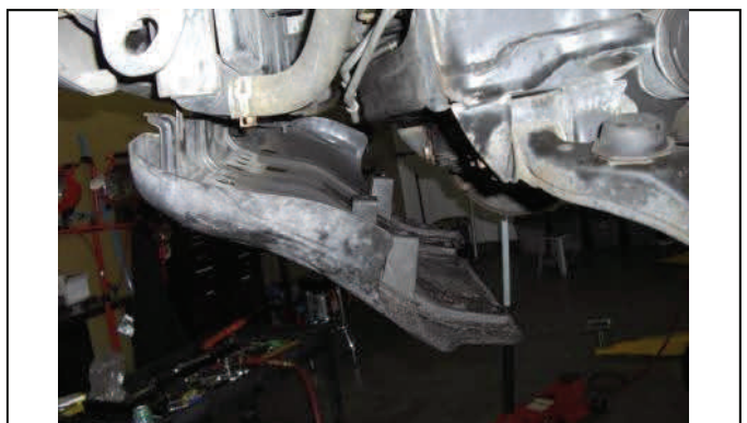
4WD models and 2.5-3.0" kits remove front skid plate
