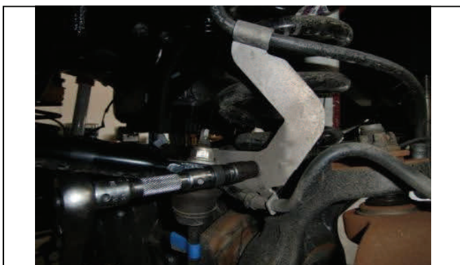
Disconnect brake line support bracket
