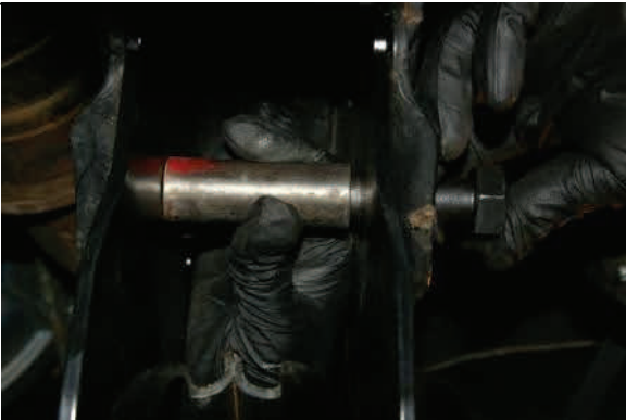
Insert crush sleeves and new hardware into drop bracket.
