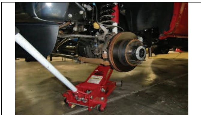
Support front axle with floor jack(s).
