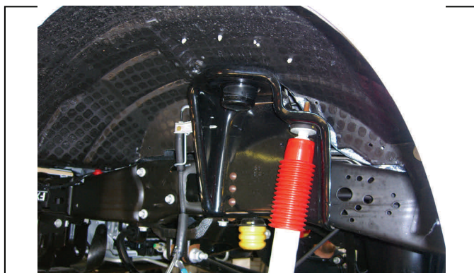
Carefully lower axle and remove coil spring
