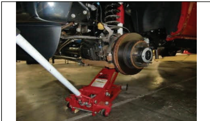
Support front axle with floor jack(s).
