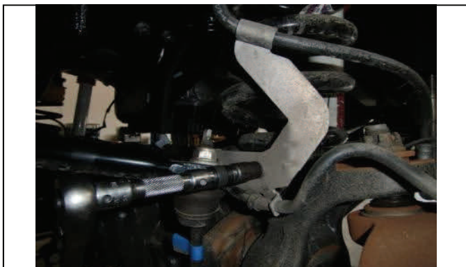
Disconnect brake line support bracket
