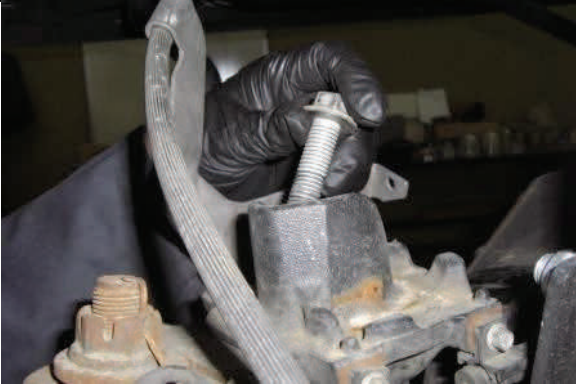
Remove bolt from middle of spring perch
