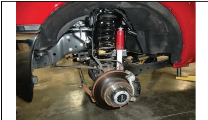
Remove front wheels and tires.
