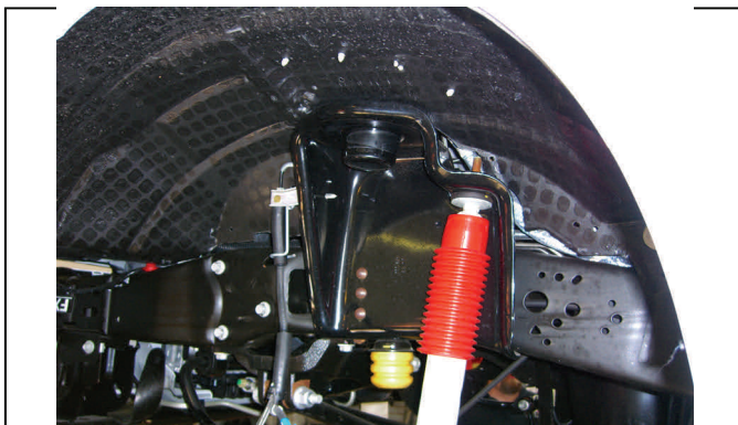
Carefully lower axle and remove coil spring
