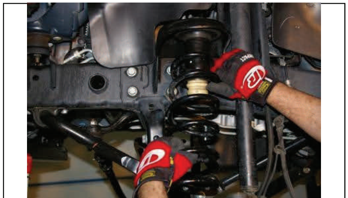
Carefully lower front axle enough to remove front spring
