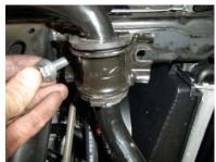
1. Remove the sway bar from the frame on both sides. Remove the metal saddle and leave the bushing.
