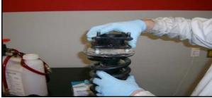
Reinstall strut into vehicle and install the new nuts provided, but do not tighten.
