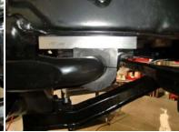
6. Sway bar spacer properly installed.
