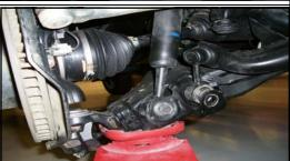
Use of a pry bar and hammer may be need to align mounting holes for the end link bolt. Install 19mm bolt and torque to factory specs.
