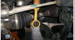
**3**. Loosen, but do not remove the 19mm lower control arm nut and bolt, Remove the 19mm lower ball joint bolts.
