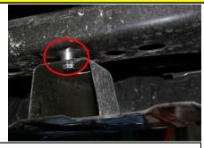
Using the hardware provided, install the M8 bolt, washer, skid plate, and 1/2 tall spacer into the back two skid plate mounting points. Use the OEM hardware for the two front mounting parts.
