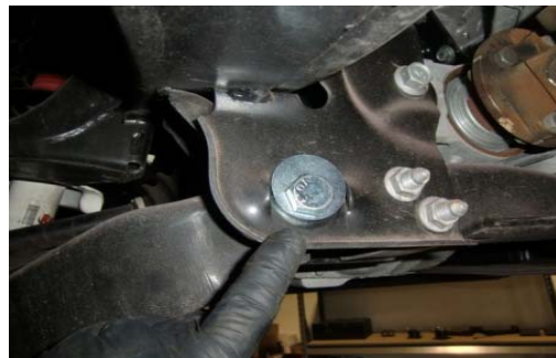
12. Install the provided alignment cam bolts as shown.
