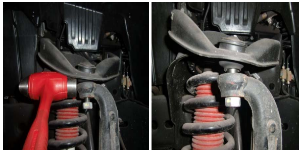
9. Separate the upper ball joint from the spindle. A hammer may be necessary.
