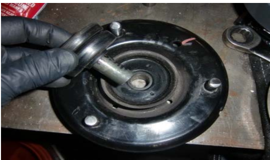
19. Remove (2) bushings and center sleeve, sleeves not reused.
