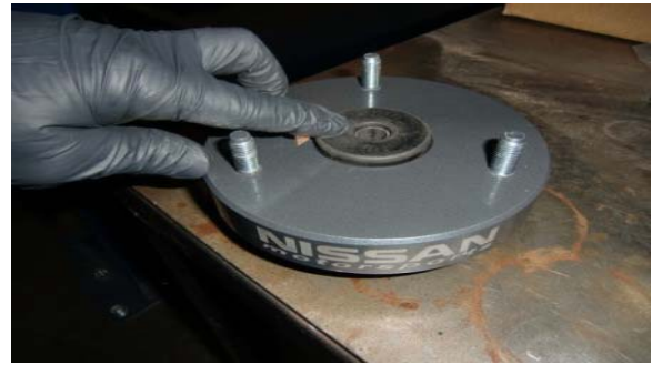
22. Insert the sleeve through the top and bottom bushings.
