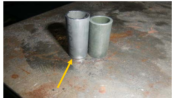
20. Important: New longer sleeve must be used.
