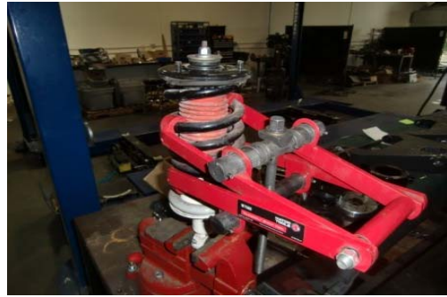
16. Use a coil spring compressor to safely remove the spring from the strut.
