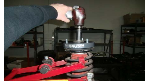
24. Tighten the OE hardware to spec.
