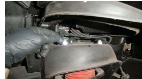
26. Install the upper strut with provided nuts.
