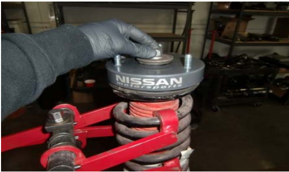
23. Reinstall the upper assembly back on top of the strut.
