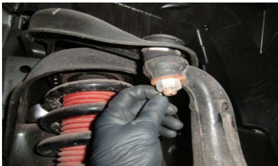
7. Remove the cotter pin from the upper control arm ball joint.
