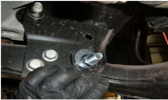
13. Tighten the alignment cam nuts in a neutral position.
