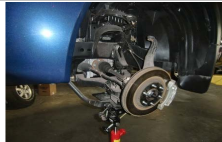
10. With the lower control arm supported, disconnect the upper control arm from the spindle, then carefully lower the jack to drop the suspension. Remove the strut from the vehicle.
