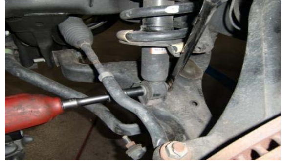
6. Remove the nut and bolt from the lower strut mount.
