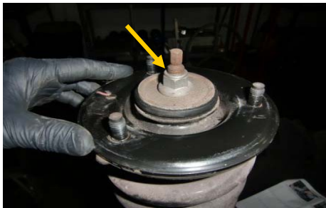
If necessary, use penetrating oil on the center stud to help with nut removal on next step. 15.
