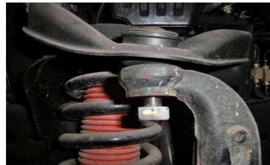
8. Loosen the upper ball joint nut, do not remove.
