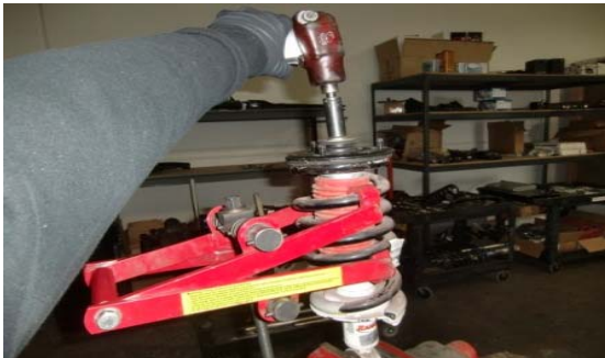
17. Carefully remove the upper coil-over center nut.
