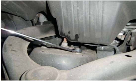
5. Remove the three upper strut nuts.
