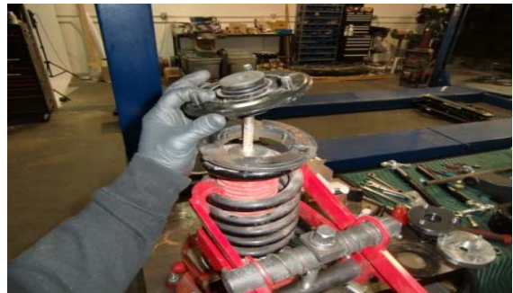
18. Remove the upper hat assembly, leave the isolator on the spring.
