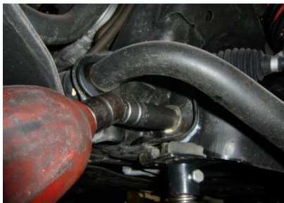
11. Remove the lower control arm bolts one at a time, to allow for installation of alignment cams.
