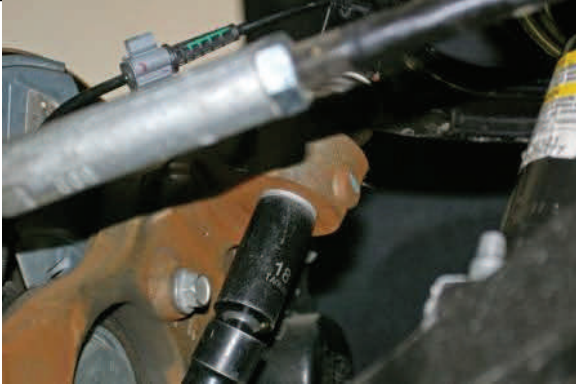
Tighten upper ball joint to spec.
