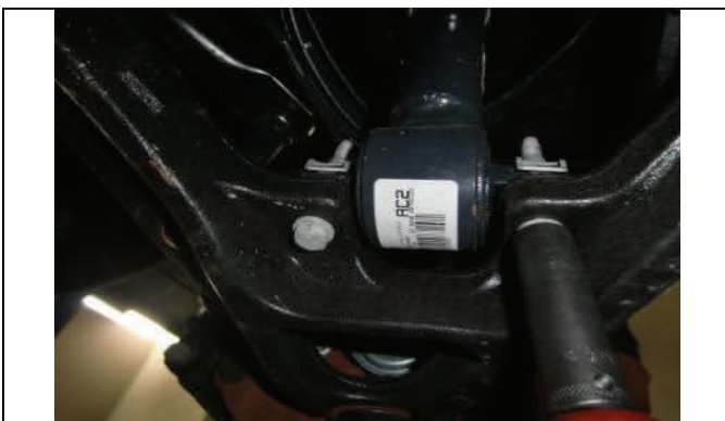
Remove lower strut mounting bolts
