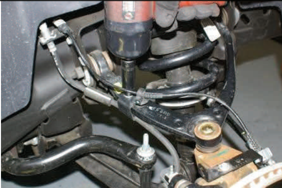
Reattach ABS/brake line bracket and sway bar end links
