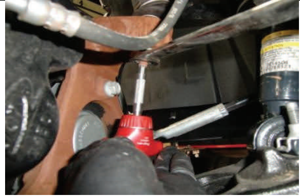
You may need to hold stud with hex key while tightening
