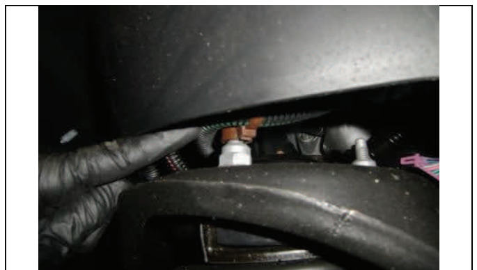
Pry up ABS retaining clips from upper strut mounting nuts
