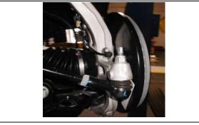
15. Reinstall the tie rods into the knuckle using a 21mm and 10mm wrench
