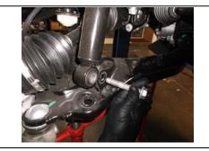
Loosen the lower control arms at the frame using a 24mm socket. Then unbolt the strut from the lower control arm using a 21mm socket.
