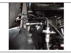
6. Remove the brake line bracket from the frame using a 13mm socket.
