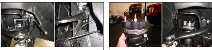
Loosen the upper control arm using a 13/16" socket and wrench. Let it rest on the droop stop, then retighten the upper control arm and torque it 11. down to 90ft lbs.
