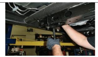
Use torsion bar loading tool and adjust new forged torsion key up just enough to allow adjuster block to be reinstalled.
