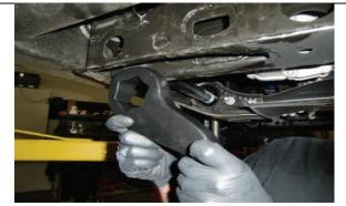
Install new 66-3011 forged torsion keys into position and slide torsion bar into hex as original.
