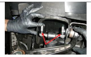
Picture shows spacers being installed onto upper studs.
