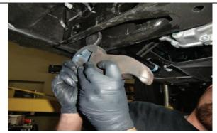
Then slide torsion bar forward in order to remove torsion key. Use caution while removing.
