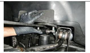
Back to the front shocks, pry down enough to allow provided spacers to be installed onto upper shock mounting studs.
