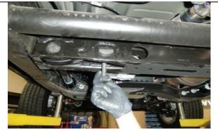
Now, install torsion key adjuster bolt and adjust for initial setting. Final adjustments will be done during alignment.
