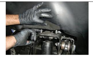
Reposition shock and tighten with new provided hardware.
