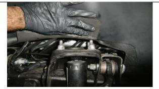
Note: To prevent damaging torsion bar tool. Peel back wheel well liner and remove (2) upper shock mounting nuts.
