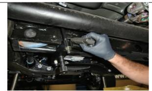
Adjust loading tool just enough to remove torsion key adjusting block from cross member. Release tool and remove.
