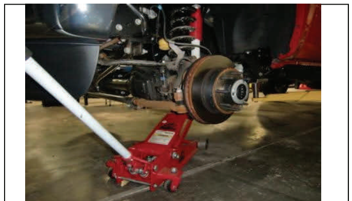
Support front axle with floor jack(s).
