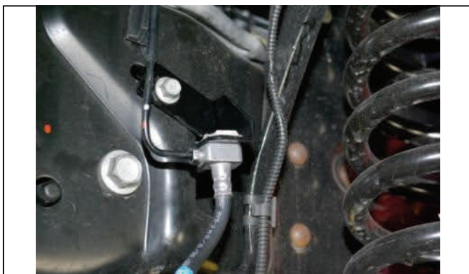
Reinstall block into bracket with retaining clip.
